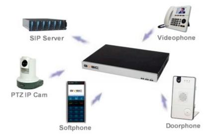
Register PTZ IP Camera; Videophone; Softphone and Doorphone to GVSC mm PBX then Videophone and Softphone users can call traditional PSTN Telephone or GSM Mobile even 3G Mobile user thru its upper layer SIP Server registration. Also 3G Mobile user can call back to PTZ IP Camera or Doorphone then open the door lock thru their Digital Out interface no matter where he is.
